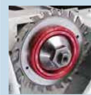
**CD** - Adjustable double scoring blade 2,8-3,6 mm, manual with motionless scoring unit
