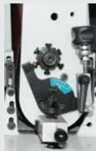
Removal adjustment system with: pneumatic rollers cutout from panel controls mechanical grit-set with 6 positions corresponding to the grains of the sand belts
