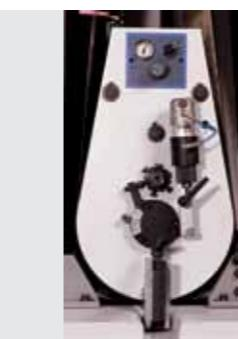
Removal adjustment system with: pneumatic rollers cutout from panel controls mechanical grit-set with 6 positions corresponding to the grains of the sand belts
