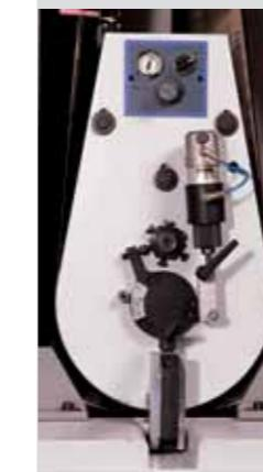
Removal adjustment system with: pneumatic rollers cutout from panel controls mechanical grit-set with 6 positions corresponding to the grains of the sand belts
